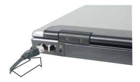
Insert the other end of the network cable into a cable modem, DSL modem, or Ethernet network jack.
